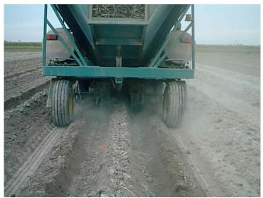
Reefsafe®/Agrispon® was applied to the plant billets as they were dropping through the planting chute. The Reefsafe®/Agrispon® rate of 1L/ha was determined by the width of the planter shoot furrow.
